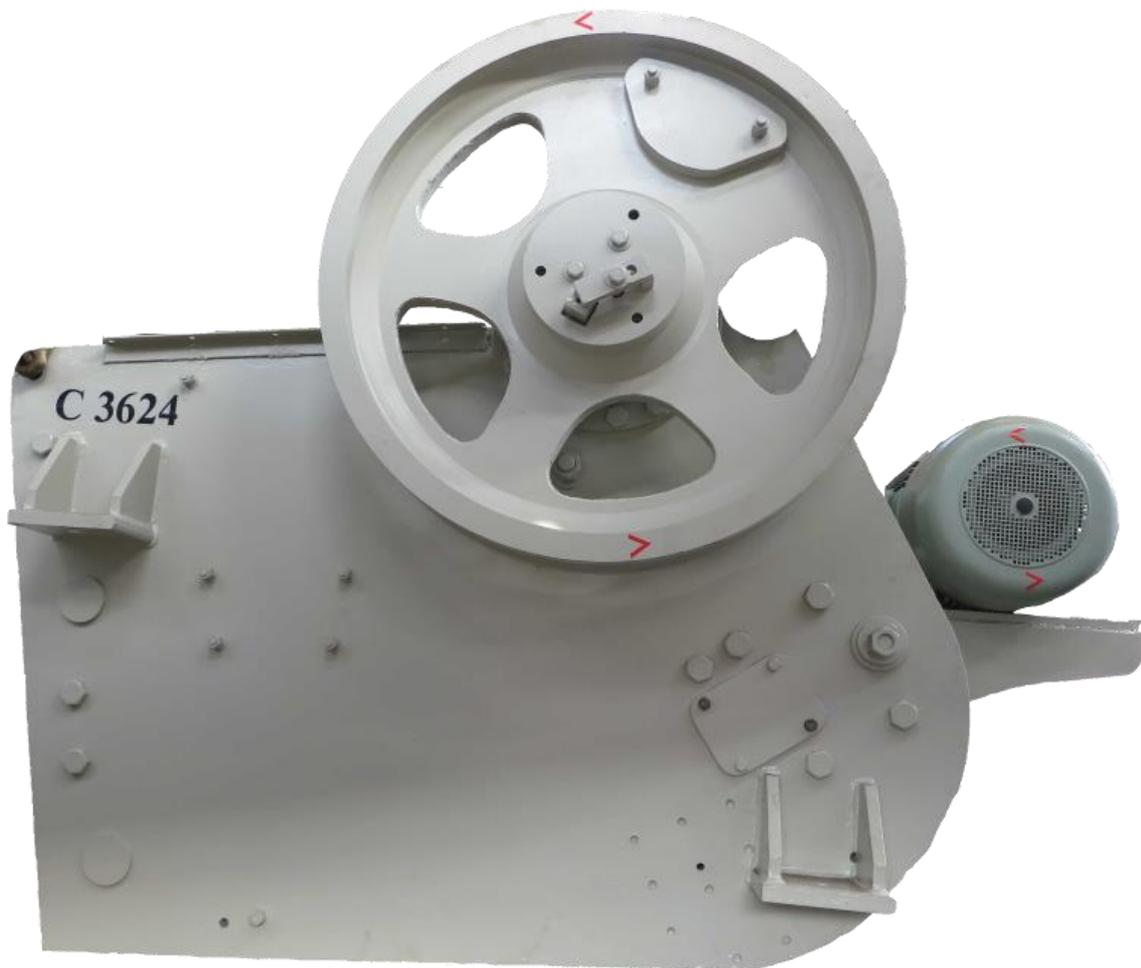
The Working Principle of Jaw Crusher is consists of many parts, like eccentric draft, frame, large belt wheel, mobile jaw, flying wheel, toggle plate, toggle plate, gap adjustment screw and so on. The main function of jaw crusher to crush large rocks into smaller rocks, gravel, rock dust and gravel to satisfy different requirements for the products.
