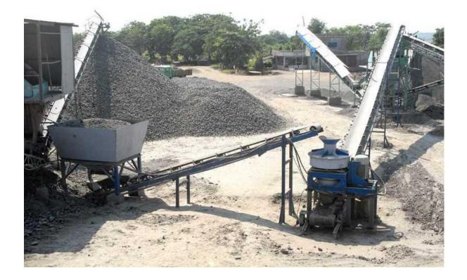
Shree Conmix Engineers Pvt Ltd. manufacturing a wide range of Vertical Shaft Impactor (VSI), which is known as "Sand Making Machine" as well as "Rubble Shaping Machine". Vertical Shaft Impactor (VSI) is used in the quarrying industries for the production of high quality aggregates & also used for production cubical sand from aggregates.
